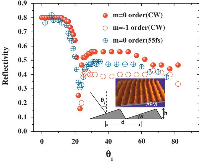
FIG. 1 (color). Sub- $\lambda$  grating diffraction;  $\theta_i$  incident angle. Inset: Atomic force microscope (AFM) image of the grating (period,  $d = 555$  nm; groove depth,  $h = 158$  nm; blaze angle,  $w = 17.45^\circ$ ).
