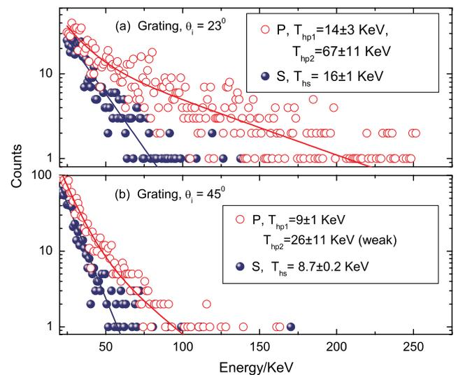
FIG. 4 (color). Bremsstrahlung spectra for the grating plasma at intensity  $I = 3.8 \times 10^{15}$  W cm<sup>-2</sup> with (a)  $\theta_i = 23^\circ$  and (b)  $\theta_i = 45^\circ$ . Solid curves denote least squares temperature fits.
