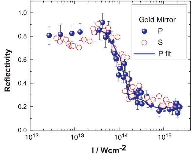
FIG. 2 (color). Gold reflectivity vs light intensity for  $s$  and  $p$  polarizations,  $\theta_i = 23^\circ$ . The knees here and in Fig. 3 correspond to plasma formation thresholds  $I_{Th}$ .
