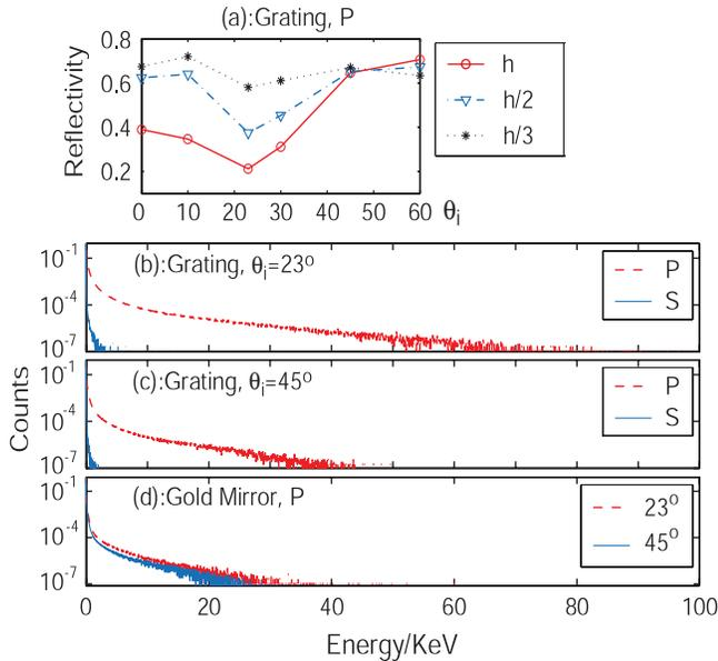
FIG. 5 (color). (a) Reflectivity as a function of angle of incidence from PIC simulation for the grating plasma with different groove depths  $h$ ,  $h/2$ , and  $h/3$ , where  $h = 158$  nm taken from the experiment. Electron energy distribution at the exit of laser pulse at (b)  $\theta_i = 23^\circ$  and (c)  $\theta_i = 45^\circ$  for the grating (groove depth  $h$ ) plasma and for the flat gold target (d).
