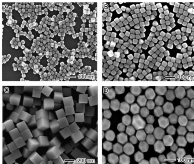
**Figure 1.** SEM images of four typical examples of Ag nanocubes: A–C) cubes 30, 50, and 200 nm in edge length and D) truncated cubes 100 nm in diameter.
