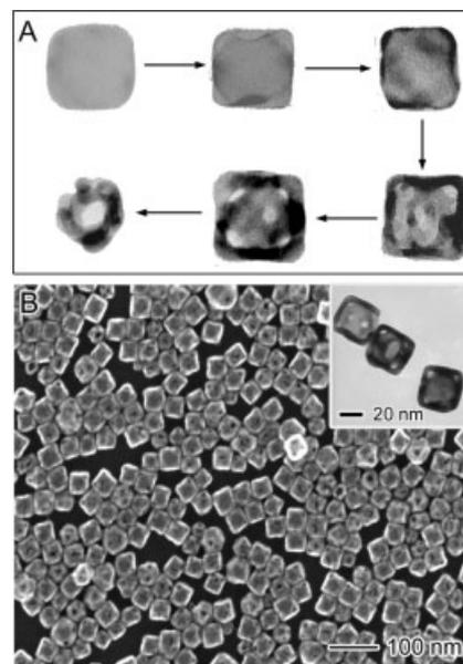
**Figure 2.** A) TEM images detailing all morphological and structural changes involved in the galvanic replacement reaction between Ag nanocubes 30 nm in edge length and  $\text{HAuCl}_4$ . B) A typical SEM image of Au nanocages derived from Ag nanocubes of 30 nm in edge length. The inset shows the corresponding TEM image.
