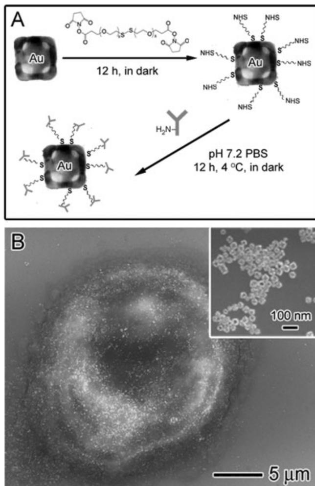
**Figure 7.** A) A schematic illustration of the two-step protocol used to conjugate antibodies to the surface of a gold nanocage. B) SEM image of an SK-BR-3 cancer cell whose surface was derivatized with primary anti-HER2 antibodies and then IgG-conjugated Au nanocages. The inset shows an SEM image at higher magnification, indicating that the Au nanocages were dispersed as a submonolayer on the cell surface.
