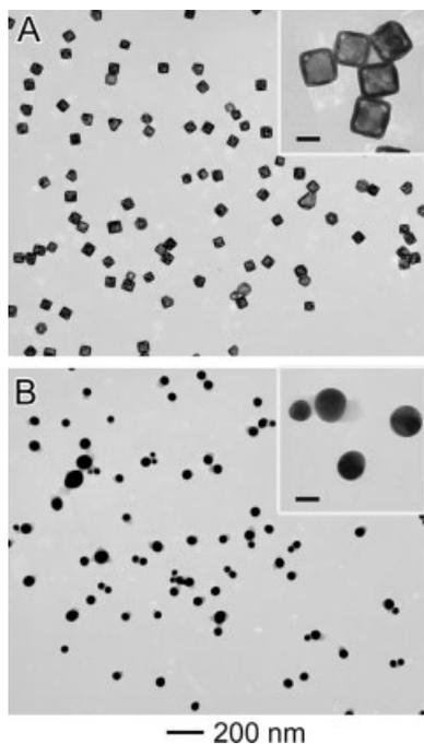
**Figure 6.** TEM images of Au nanocages (55 nm in edge length) A) before and B) after exposure to a camera-flash light. The insets are the enlarged TEM images, with the scale bars being 50 nm. Note that the nanocages melted and became spherical droplets due to the photothermal effect.
