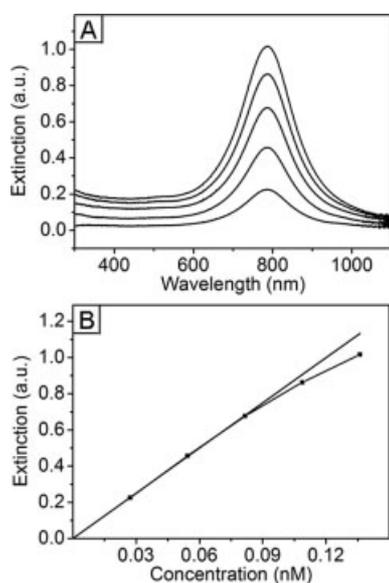
**Figure 4.** A) Extinction spectra of the Au nanocages shown in Figure 2B, which were prepared as dispersions of different concentrations. B) A plot showing the dependence of peak extinction on the concentration of Au nanocages. Note that the data points (■) deviate from the linear fitting when the concentration was higher than 0.09 nM.
