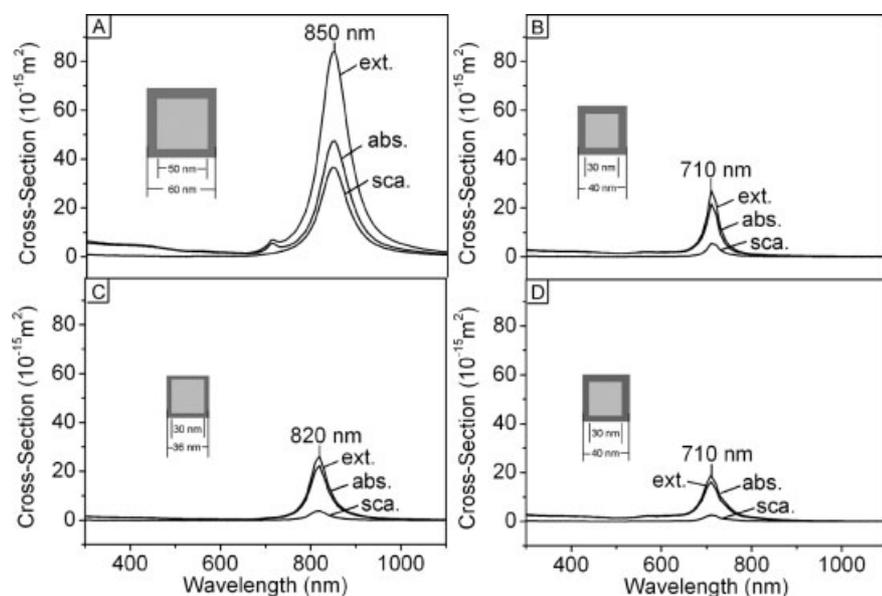
**Figure 5.** Extinction spectra calculated using the DDA method for Au nanocages having four different sets of geometric parameters: A) a Au nanobox 50 nm in inner edge length and 5 nm in wall thickness; B) a Au nanobox 30 nm in inner edge length and 5 nm in wall thickness; C) the same as in (B), except that the wall thickness is 3 nm; and D) the same as in (B), except that the eight corners are decorated with triangular holes 5 nm in edge length.
